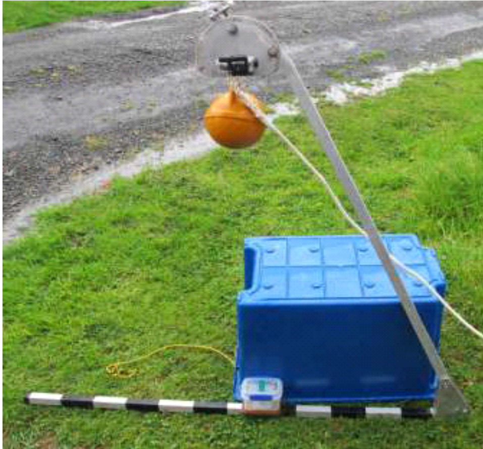
Figure 5: Baited underwater video (BUV) apparatus with GoPro camera mounted at top facing the baitbox on the bottom bar. Also note the 10cm spaced scale along the bottom bar and the pressure resistant float attached at the top.
