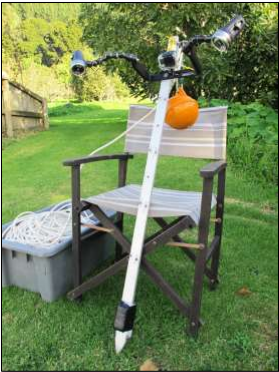
Figure 4 GoPro drop camera system.
