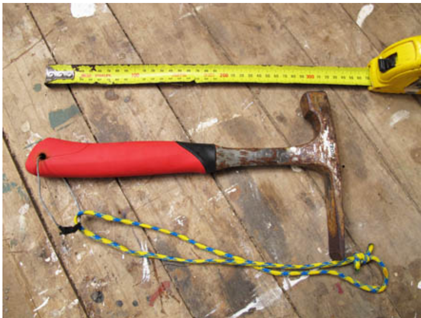
Figure 20 The preferred hammer with a chisel-shaped end, note safety string, normal practice in diving is that all tools need to have a way to be attached to the diver or can be attached quickly to allow the diver to have his hands free in case issues arise with the diving equipment.
