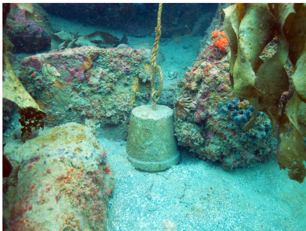
Figure 6 An example of an anchor block for marking the seaward corners of the management trial areas
